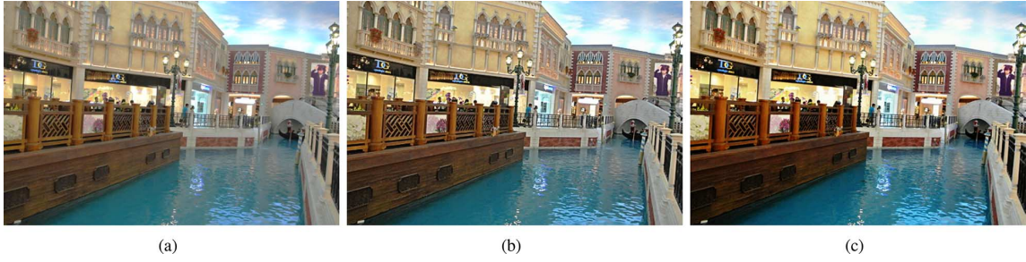
Fig. 14. Contrast enhancement results comparison (insufficient enhancement case). (a) Test image; (b) enhanced image with NoG = 1 ; (c) enhanced image with NoG = 3 .
