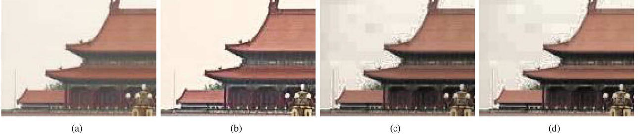
Fig. 10. Demonstration of the blocking artifacts in contrast enhancement (cropped for visualization). (a) Input image; (b) enhanced image with proposed method; (c) HMF output; (d) RSIHE output.
